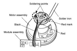
1. Remove the two soldered module assembly lead wires to the motor assembly terminals.
