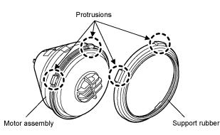
1. Remove the support rubber from the motor assembly.
