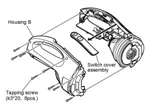
1. Remove 8 housing tapping screws and remove the housing B and the switch cover assembly.
